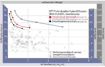
Oxygen transfer efficiency data from independent test institutes with full-floor coverage of basin. Complete test reports available on request.
