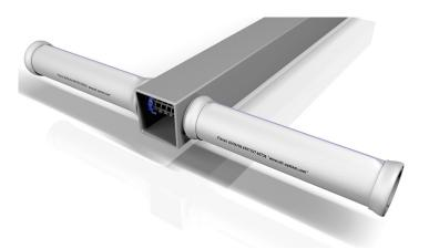
**STANDARD 2** diffusers are installed quickly and easily on rectangular headers with 40 or 45 mm (1.57" or 1.77") diameter outlet openings. They are installed in pairs using double-threaded connectors available in engineering plastic PP-GF or VA-grade stainless steel.
