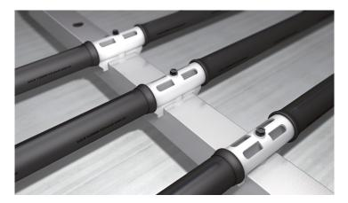
**MAGNUM**<sup>®</sup> diffusers can be installed on rectangular or round headers with 30 mm or 38 mm (1.18" or 1.50") outlet openings. We offer connectors for DN 80, 100 and 125 mm (3.15", 3.94" and 4.92") diameter round headers and 80, 100 and 120 mm (3.15", 3.94"and 4.72") rectangular headers.
